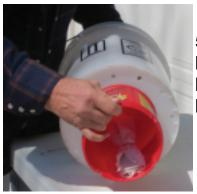
5. Thread the bundled dishcloth through the 1 3/4" hole in the center of the bucket and coffee can. The bottom of the coffee can should touch the bottom of the bucket.
