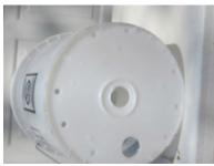
3. Turn the bucket up-side-down. Using the 1 3/8" hole saw, drill one hole approximately one inch from the edge of the bucket.
