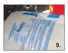
9. Remove the top assembly (top bucket, towel & coffee can) from the bottom 5 gallon bucket. Using the 3/8" drill bit, drill an overflow hole just above the point you marked on the bottom bucket. (The point at which the inner 5 gallon bucket rests on top of the coffee can).
