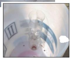
lowest bottle resting in the 1 3/8" hole drilled in the top bucket during Step 3. Bottles do not need to be secured, but if desired use duct tape or non-toxic glue to fasten bottles together. Bottles should reach the top edge of the top bucket.
